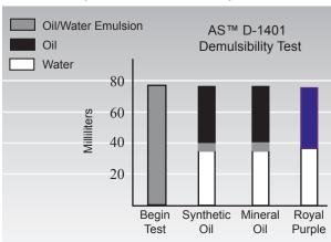
Royal Purple Synthetic Oil with Synerlec ™ separates rapidly from water to remain dry. Dry oil greatly extends bearing lige. Water is easily drained from bottom of oil reservoir.
