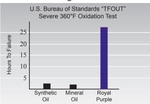
Royal Purple is 10 times more oxidation stable in this test. In the U.S. Steel/AS™ D-2893 lab test, results equated to a 20 year oil change interval in field service (271 days in test with 0% viscocity increase). Unless oil is contaminated, oxidation is the sole measure of oil life.
