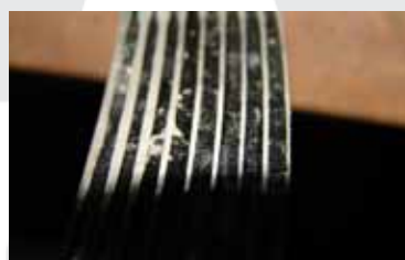
Incorrectly rolled-in grooves with laminated cutter
